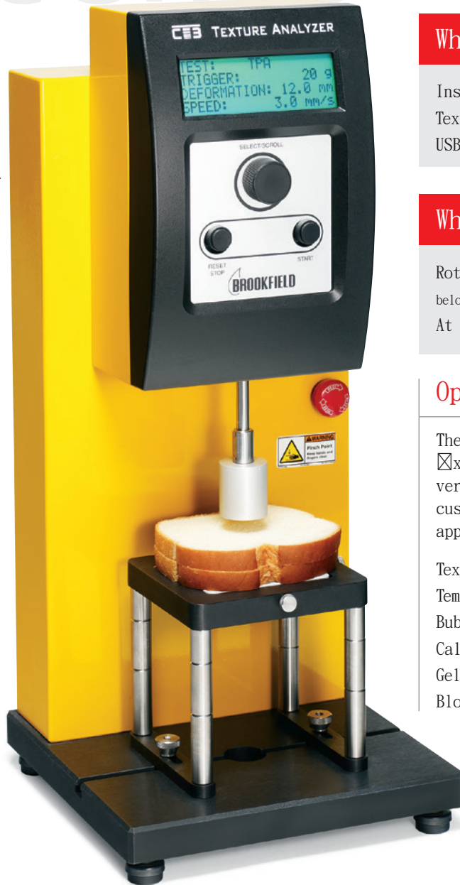
CT3 with Fixture Base Table and Cylindrical Probe in compression (TPA) mode
