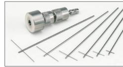
The Helipath Stand is supplied with a set of six T-bar spindles that attach to the instrument with a special coupling.
