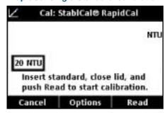
In the range up to 40 NTU, the single standard RapidCal calibration mode reduces calibration complexity by eliminating multiple standard full calibrations. You save time and ensure you meet reporting requirements.
