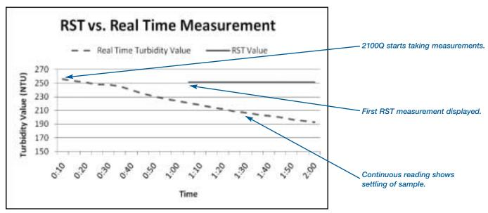
Although the sample continuously settles out of solution, the RST calculated value does not change. No more guessing and no more replicate runs
